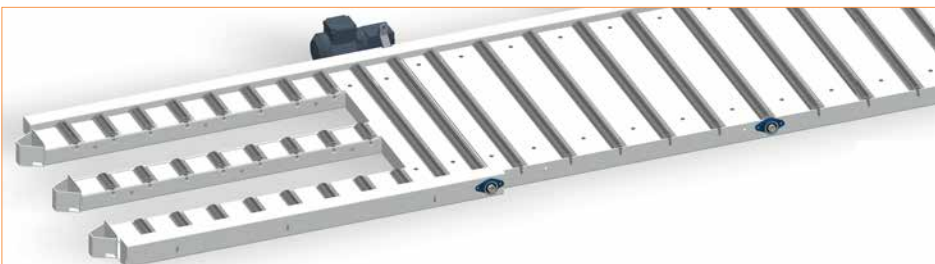
Conveyor for deposit / reclaim
